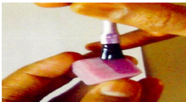
Fig 10: Application of tray adhesive on the test sample
