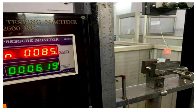
Fig 11: Debonded test sample on Universal Testing Machine
