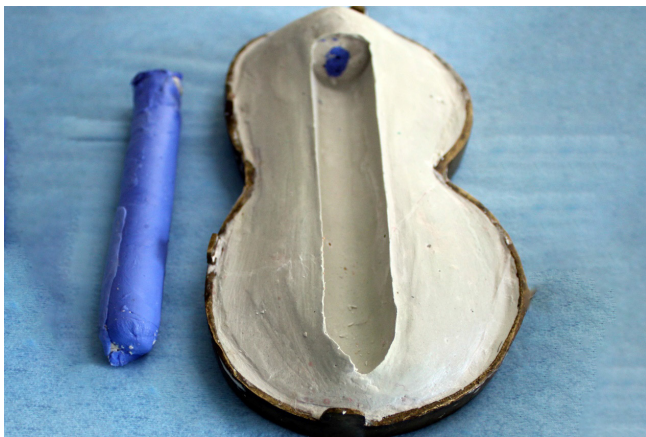
Fig. 7. Retentive base within the investment material after dewaxing.
