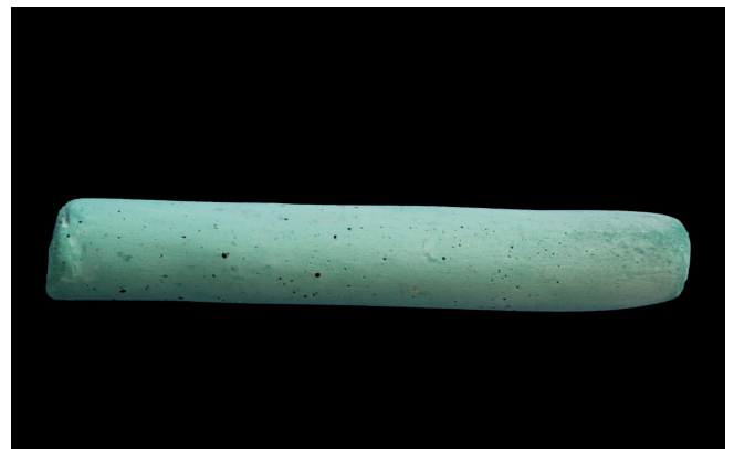
Fig. 2. Cylindrical mold made of type III dental stone.
