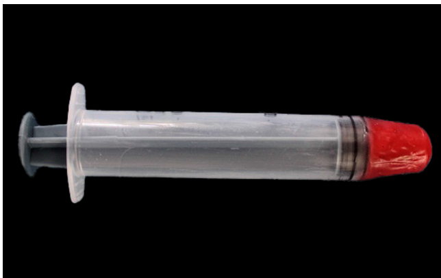
Fig. 1. Syringe tip molded with wax.
