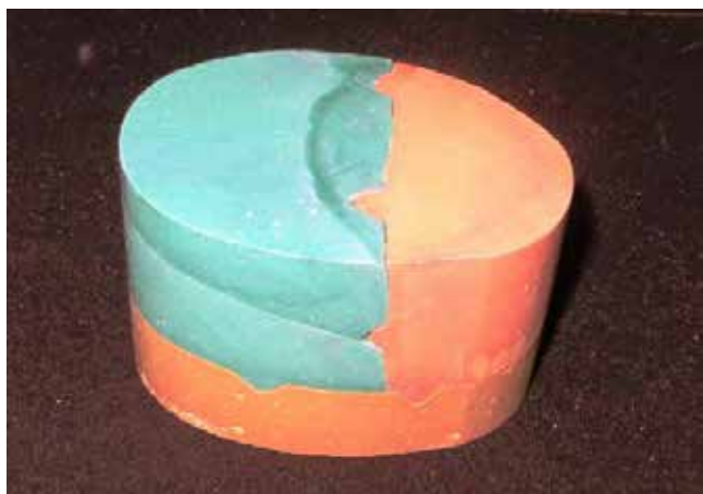
Fig: 6 b ; Three piece mould
