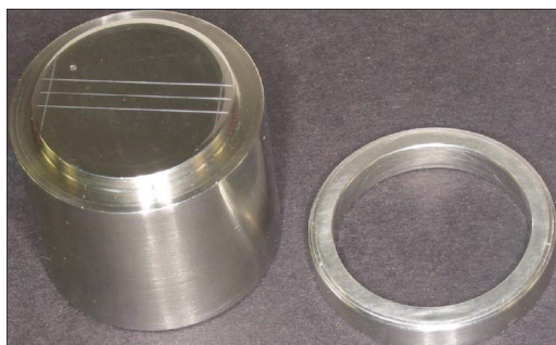
FIGURE 1: Stainless steel die with ADA specification no: 19
