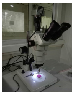
FIGURE 4: Stereo microscope (MAGNUS) used to evaluate the dimensional accuracy and surface detail reproduction of sample
