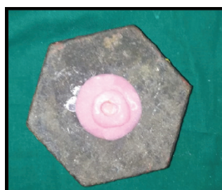
Fig 13. Modification of the 2kg weight with acrylic resin
