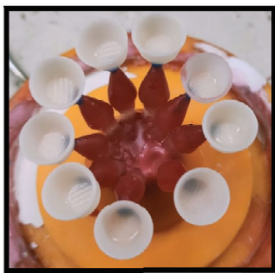
Fig 9. Sprues attached to the 3D printed resin patterns
