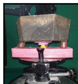
Fig 14. Standardized pressure application for obtaining silicone replicas
