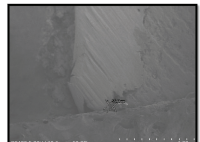
Fig 18. SEM imaging to measure marginal gap
