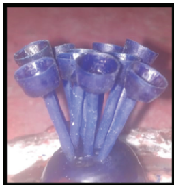
Fig 5. Sprues attached to the crucible former
