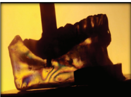
Fig 4: Strain patterns in short implants under axial loading
