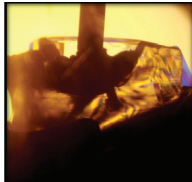
Fig 5: Strain patterns in conventional implants under oblique loading
