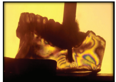
Fig 3: Strain patterns in conventional implants under axial loading
