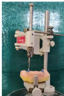
Figure 12 & 13. A surveyor used to ensure parallelism between the studs.
