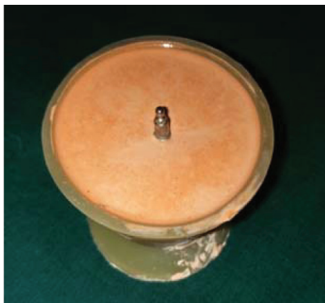
Figure 5. Implant placed in Type IV Dental stone
