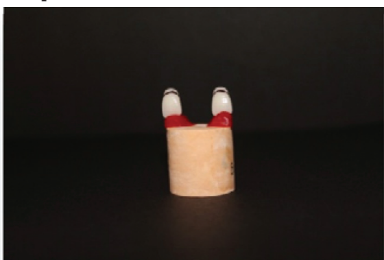
Fig 1 Bonding surface area of the denture tooth was demarcated and standardized in all 4 groups
